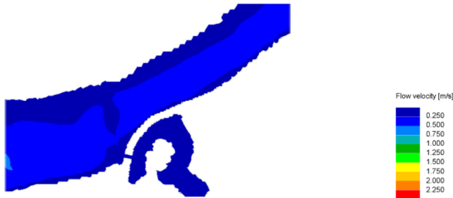
Fig. 4.3 RSim-3D results – Submersed Guiding Wall – CP02 – surface near flow velocity – Q1940 \text{ m}^3\text{s}^{-1}
