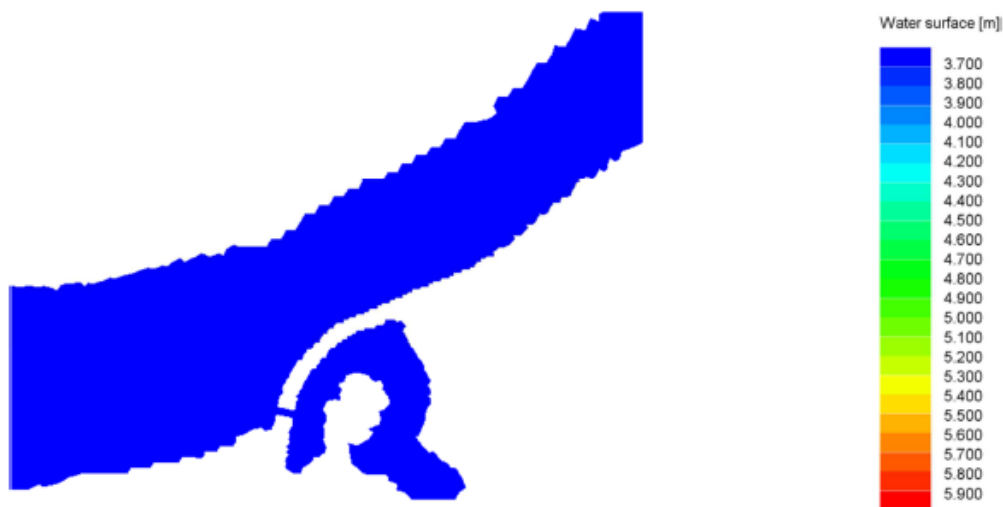
Fig. 4.1 RSim-3D results – Submersed Guiding Wall – CP02 – water surface (m a.s.l.) – Q1940 \text{ m}^3 \text{ s}^{-1}
