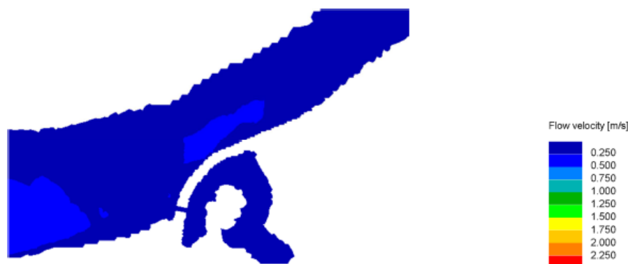
Fig. 4.4 RSim-3D results – Submersed Guiding Wall – CP02 – bottom near flow velocity – Q1940 \text{ m}^3\text{s}^{-1}
