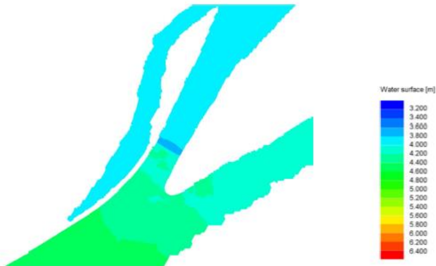
Fig. 3.1 RSim-3D results – Sill Bottom 0 B.S.C – CP01 – water surface (m a.s.l.) – Q1940 \text{ m}^3 \text{ s}^{-1}
